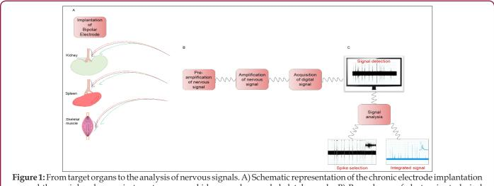
around the peripheral nerve in target organs as kidneys, spleen and skeletal muscle. B) Box scheme of electronics technical setup. C) Detection and analysis of nervous signal by the selection of spikes and the integrated signal.
