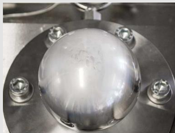
Figure 2: Inflated test specimen without black & white pattern close to failure. Stress whitening can be observed. Photo: Fraunhofer LBF.
