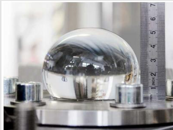
Figure 1: Inflated test specimen without black & white pattern, applying the orifice of the Ø50 mm diameter. Photo: Fraunhofer LBF.
