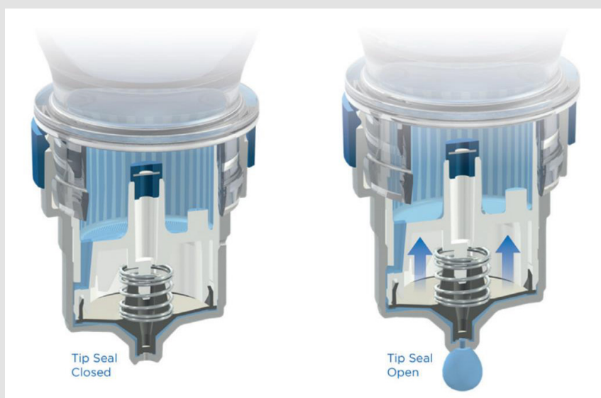
Figure 4: Aptar Pharma’s Ophthalmic Squeeze Dispenser. Image taken from aptar.com [35].
