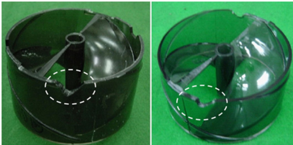
Figure 4: Fractured parts from the field and ALT. (a) Failed products returned from the marketplace. (b) Fracture after first ALT.
