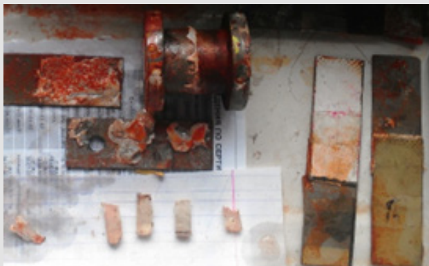
Figure 3: Image of epoxy composite samples, coatings and glued steel plates and cylinders.
