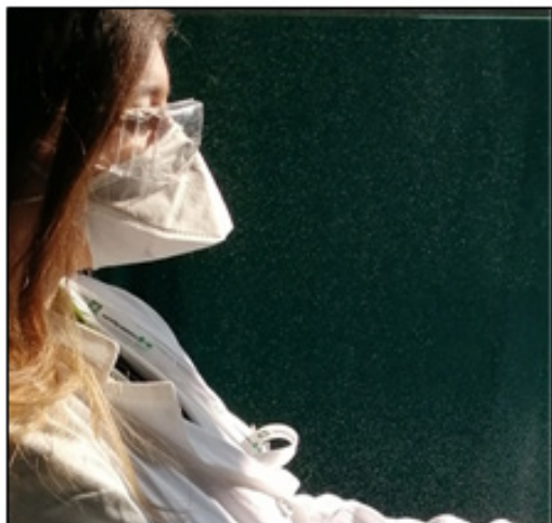
Figure 5: Qualitative fit testing. The test agents were areodispersed in the air by a nebuliser.
