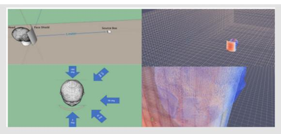
Figure 1: Simulation Setup, Discretization (Meshing), and Angles of Attack.
