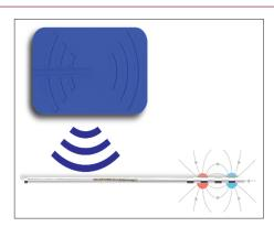
**Figure 2:** Neurostimulator receiver. The contacts on the electrodes are managed by independently integrated, circuits that are application specific. The circuitry system within the device produces charge-balanced waveforms.
