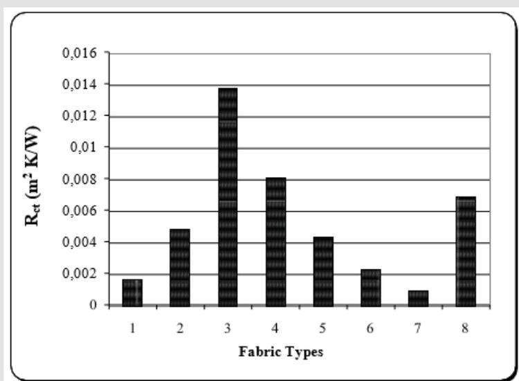
Figure 14: Thermal Resistance results of the fabrics.
