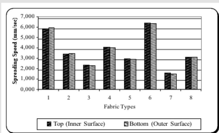
**Figure 11:** Spreading Speed (mm/sec) values for the fabric.
