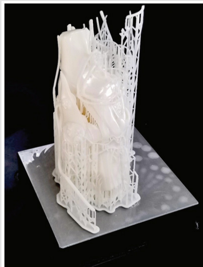
Figure 6: 3D print of knee joint with scaffolding (bones, connective tissue, arterial and venous systems, nerves) in Formlabs White V4 Resin.
