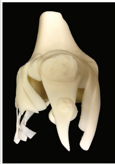
Figure 9: Anterior view of femoral segment of knee joint (bones and connective tissue) in Formlabs White V4 Resin.
