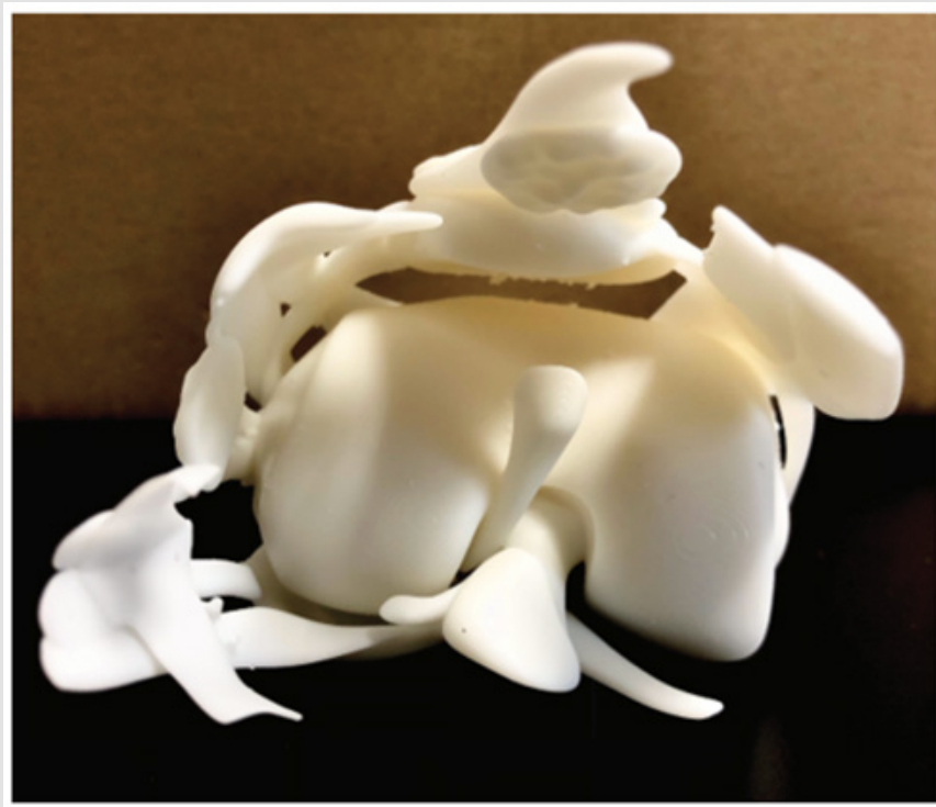
Figure 10: Inferior view of femoral segment of knee joint (bones and connective tissue) in Formlabs White V4 Resin.
