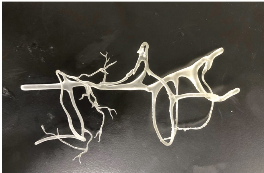
Figure 4: Arterial system surrounding the knee joint printed in Elastic 50A Resin.
